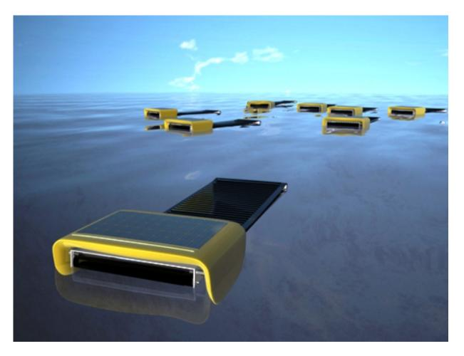
Seaswarm is pretty similar to Ocean Therapy Solutions' device which filters crude oil from sea water, because it is designed to specifically siphon crude oil from sea water at a spill site. Ocean Therapy Solutions' largest device could siphon up to 200 gallons a minute, but Seaswarm claim that as a collective group, their machines can work together to clean even larger areas of ocean. ( $\pi\epsilon\rho\iota\sigmaooter\rhoa...$ )
